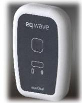
Where two people wearing an eqWave device infringe a pre-configured distance from each other the device will alert the wearers to remind them to separate and record the infringement for contact tracing. (No personal data is recorded)
