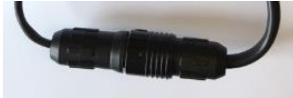
Figure 9 Sensor Belt ancillary connector mated to external sensor
